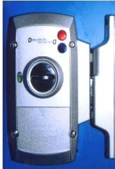
Close the door to see if the closing sensors will work normally after inserting a latch between the inside unit and the door frame. In case there is a wide gap, adjust the gap using the provided latch supporter.
