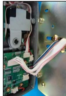
Insert the batteries into the inside unit and connect the main P.C.B. Connect cable and Fingerprint Module connect cable of the outside unit to the inside unit.
