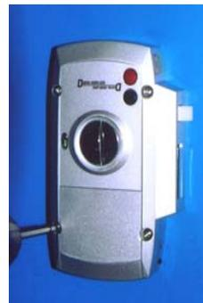
Tighten the two bolts to fix the inside unit and the steel plate in a diagonal direction. Confirm that the numeric button, start switch and motor are working normally. If they are not working normally, check the cable. Otherwise, tighten fully the rest of the bolts.
